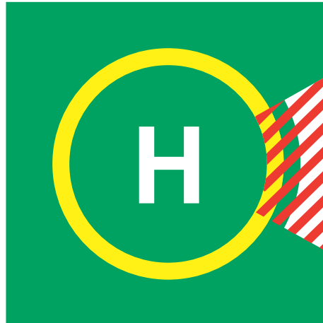
Figure 5-5. Helideck prohibited landing sector marking
