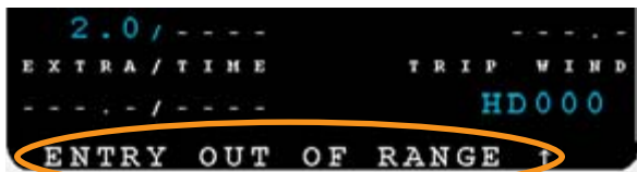
Figure 2: MCDU scratchpad message for ZFW range check
