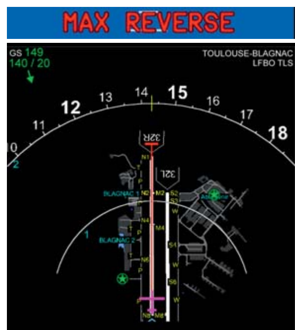
Figure 6: Illustration of PFD and ND (ARC mode in Airport Navigation range) in case of ROP alert
