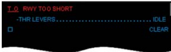
Figure 9: ECAM alarm when the Lift-off Run check detects a risk of overrun at take-off (take-off power condition is true)
