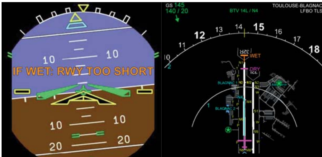
Figure 3: Illustration of PFD and ND (ARC mode in Airport Navigation range) in case of “Wet” ROW alert
