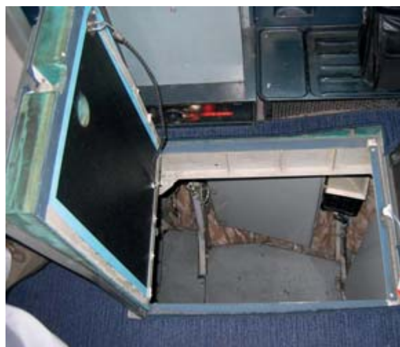
Figure 2: Open access hatch seen from behind the first officer's seat
