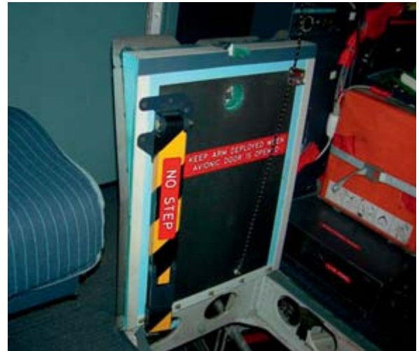
Figure 3: Avionics access hatch with folded protective arm
