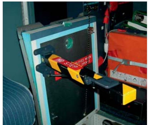
Figure 4: Avionics access hatch with unfolded protective arm
