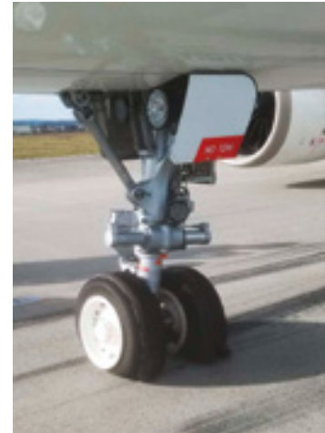
(fig.3) View of the NLG after landing
