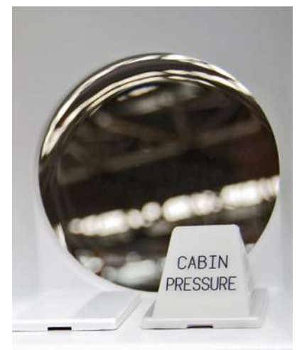
(fig.2) Cabin door with the residual pressure warning light
