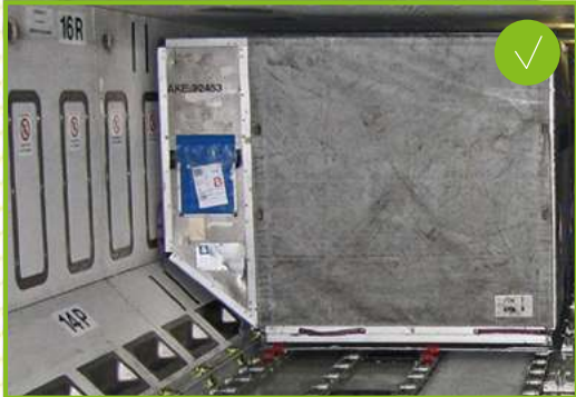
Don't load out of contour ULDs (containers or pallets)
