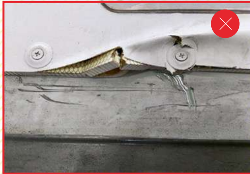
Don't load out of contour ULDs (containers or pallets)
