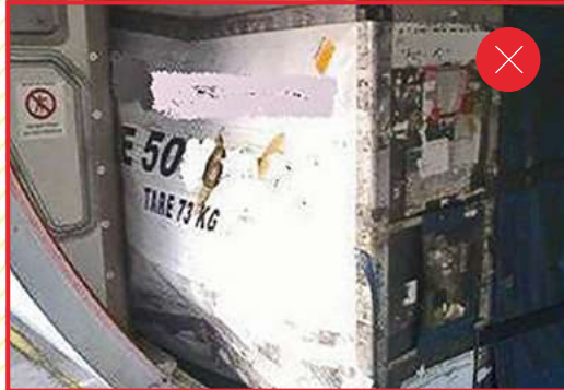
Don't load out of contour ULDs (containers or pallets)
