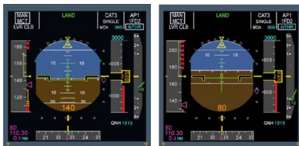
Figure 1 PFD (at 140ft and 80ft) after setting MCT instead of TOGA at 200ft during an ILS approach, (symbolic graphic – no direct reproduction of the described events)
