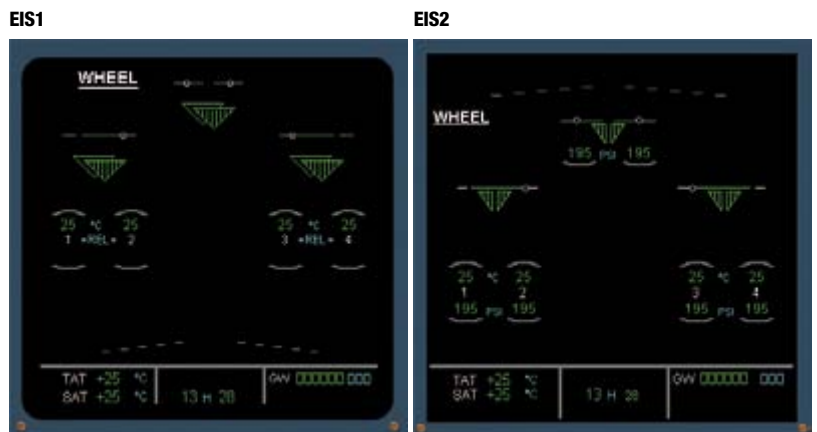
Figure 2 EIS 1 versus EIS 2 WHEEL Systems Display Page
