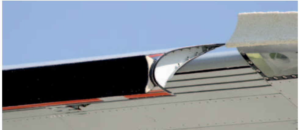
Figure 1 Polystyrene shapes simulating ice accretion
