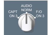
Figure 3 Audio Switching rotary switch
