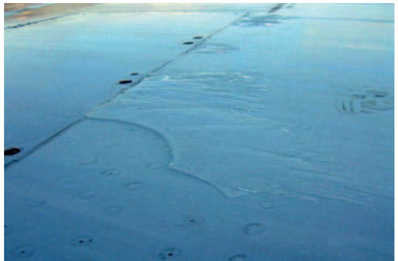
Figure 2 Clear-ice contamination on the wing
