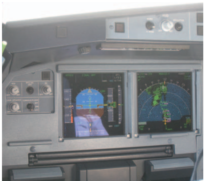
Figure 6 The RNP trajectory on the A319 Navigation Display leading to runway 12 at Vágar. Notice the lateral and vertical deviation indicators (L/DEV and V/DEV) on the Primary Flight Display.
