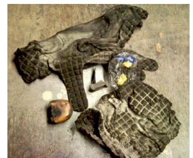
Figure 2 Foreign objects found in an APU compartment
