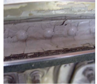
Figure 12 Corrosion between the interlocking surfaces of aerial connections could lead to loss of communication
