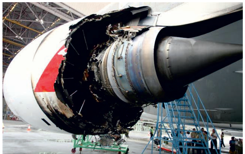
Figure 2 QF32 n°2 engine after it sustained an uncontained failure of the Intermediate Pressure (IP) turbine disc
