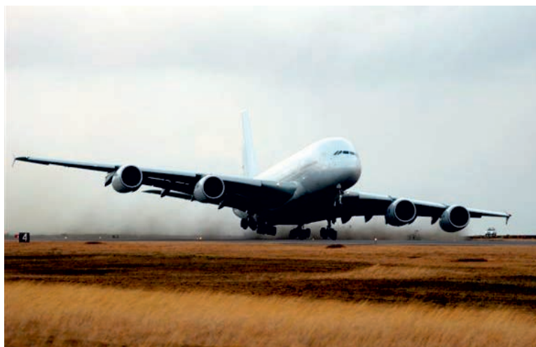
Figure 1 Take-off from Keflavik, Iceland. Note how the wind lifts the right wing. Maximum reported crosswind at the time was 56 kt in gusts
